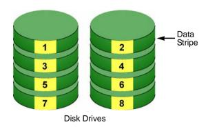
Figure 1. RAID 0 Striping interleaves data across multiple drives
